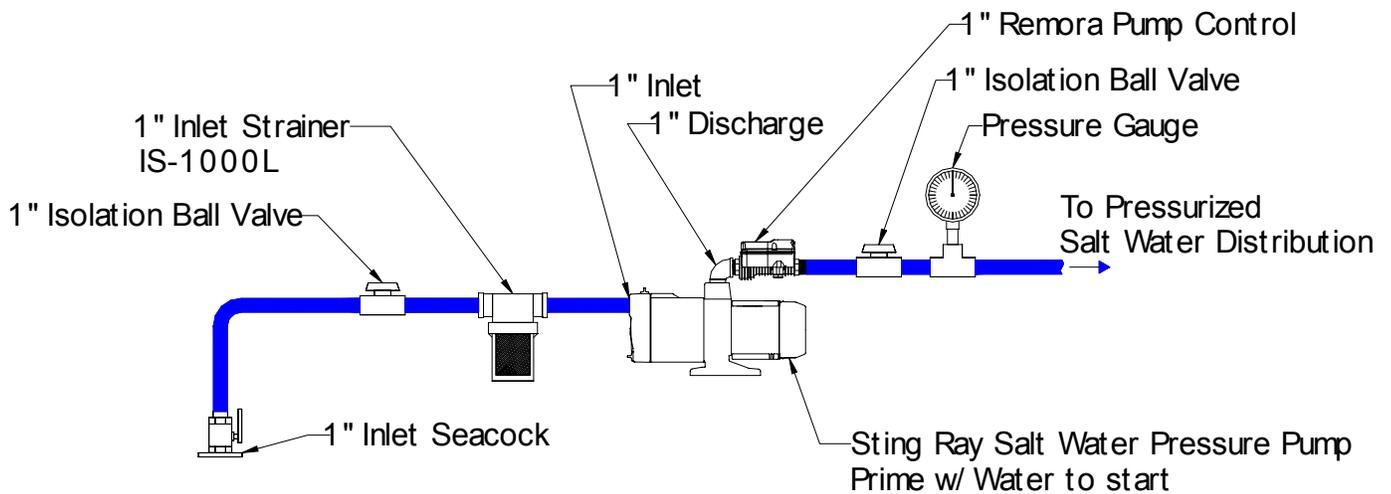
1. Secure pump on level platform. Failure to comply may affect the ability of the pump to prime itself.
